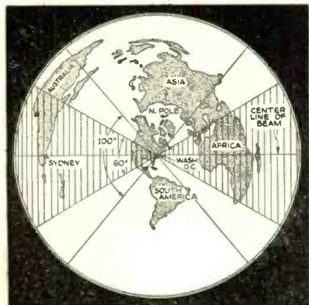
Figure 2. Approximate coverage of a 2-section flat-top beam at Washington, D. C., with the maximum response centered on Sydney, Australia. This direction is broadside to the antenna. The antenna itself runs approximately north and south (more exactly 8° W. of N. and 8° E. of S.). The shaded area indicates the angle over which maximum improvement is obtained.
