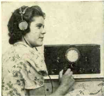
Front view of 6-tube Superhet.
